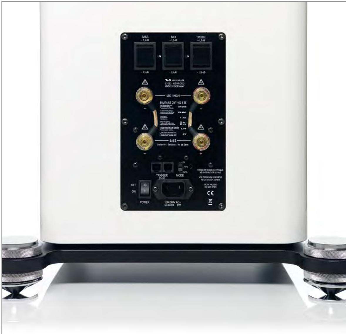
All SOLITAIRE® models are fitted with level adjusters for the mid-range and electrostatic drivers. Instead of modifying the frequency response, the adjusters alter the loudness level of the drive units. This makes it possible to fine-tune each loudspeaker individually to suit its position in the room, thereby largely eliminating problems associated with their location.
