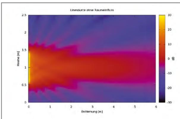
The graph alongside shows the radiation behaviour of a Line Source - such as the electrostatic driver used in the CWT 1000-8 SE - without the influence of a room. Interference effects produce a homogeneous, cylindrical, axial sound dispersion pattern in front of the loudspeaker, whose intensity does not diminish even over quite a long distance.
