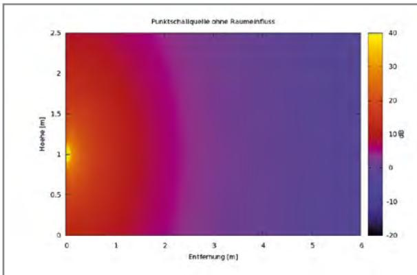
The graph alongside shows the radiation pattern of a point sound source such as a cone loudspeaker, without the influence of a room. There is nothing to impede the sound's radiation, and its dispersion pattern is virtually spherical. Sound intensity diminishes relatively quickly, since the radiated energy is distributed throughout the whole available volume.
