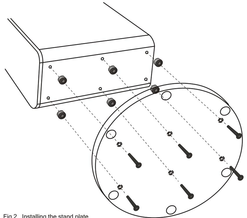
Fig 2. Installing the stand plate
