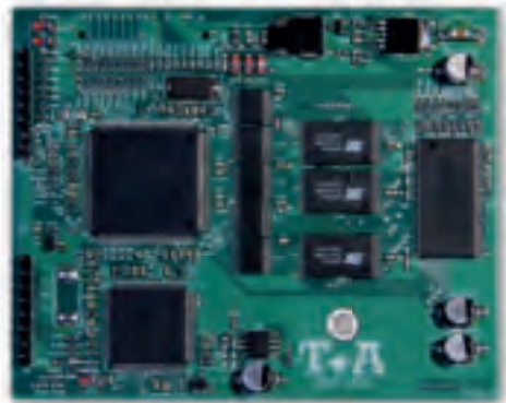
The high definition surround decoder with two Dual-Core 56 Bit DSP's is also the latest and most up-to-date of its kind.
